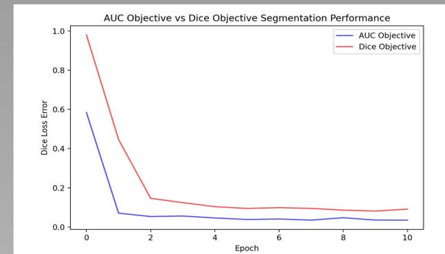
Figure 5 - Loss Performance With Dice and AUC Objectives (Dice Coefficient)
