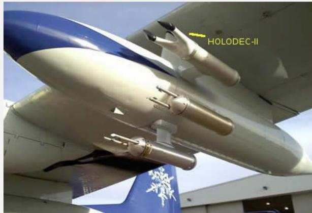
Figure 1 - HOLODEC-ii Hydrometeor Detector
