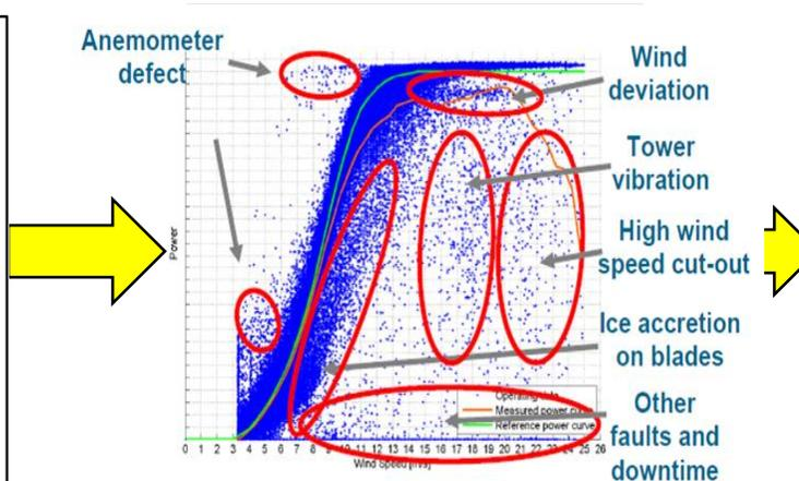
Predict **wind energy** of each turbine using manufacturer or empirical power curve algorithms
