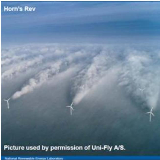
**Turbine wakes result in power loss, turbulence, wind shear and overall wear and tear on the turbines drive trains**
